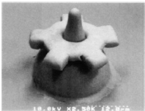
Figure 52. Micro gear-wheel affixed to a shaft. The gear wheel is freely movable. Reprinted with permission from ref 605. Copyright 2000 Optical Society of America.
